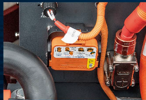
External service switch Easy to operate Effectively prevent electrified misoperation
