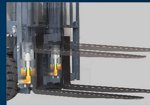
Standard mast up and down buffer, avoid extreme impact, intelligent safety
