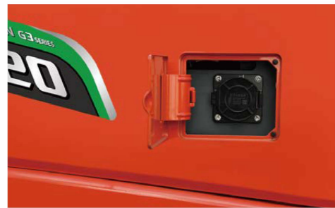
National standard fast charging port supports up to 200A fast charging
