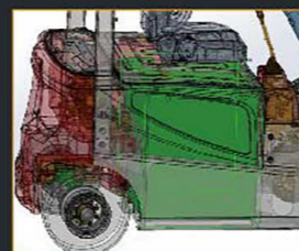
Middle and sink layout of the battery
