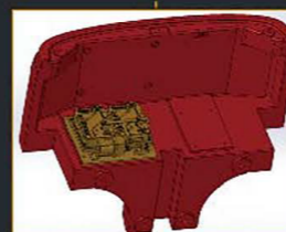
The electric control is placed on the counterweight
